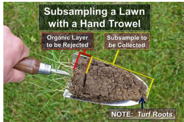
Figure 8: Hand trowel for soil sampling. The organic layer will be explained in the section below on sampling tips. Photo by Turf Roots.
